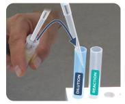
Add 100  $\mu$ L of clarified sample extract to the dilution tube and mix thoroughly with pipette tip.
