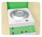
Immediately remove a portion of the extract and centrifuge for 30 seconds at 2000 x g (NOT RPM).
