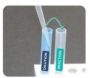
With a **new** pipette tip, transfer 100 µL of the diluted sample extract to the reaction tube and mix thoroughly with pipette tip.
