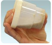
Immediately shake vigorously for 10 seconds by hand to ensure proper wetting, then shake an additional 1 minute on mechanical shaker (or by hand for 2 minutes).
