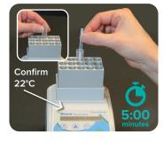
Place reaction tube in Incubator and acclimate for 2 minutes\* before adding TotalTarget Gluten Strip; wait **5 minutes** for results.
