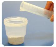
Add 75 mL of 1X Grain Extraction Buffer to the 25 gram sub-sample and cap tightly.
