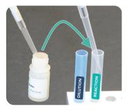
With a **new** pipette tip, add 100 μL DB2 Buffer to clean reaction tube.
