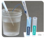
To a blue dilution tube, add 200 µL of distilled, deionized or bottled water.
